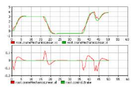
The above figure shows the diagrams for the variables **PosCar**, **PosLoad**, **Angle** and **Brake**. As follows from the diagram the brakes are not activated during operation. Thus the brakes activating condition may be too strict.
