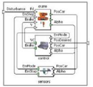
The crane object consists of the crane- mechanics and the DC-motor. The mechanics of linear and nonlinear systems, as well as the DC-motor were implemented plainly using given equations. The control block generates voltage for the mo-
