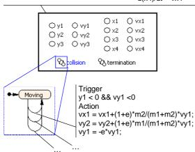
The hybrid statechart can be entered in AnyLogic model editor, and the simulation engine automatically detects change events, changes the working set of equations and readjusts the numerical methods.
