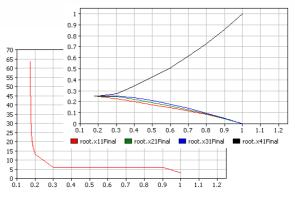
Task c1: Boundary value problem. A binary search was implemented within AnyLogic environment as Java script. AnyLogic obtains the value of e = 0.5874011 with the precision set to 1e-7.
