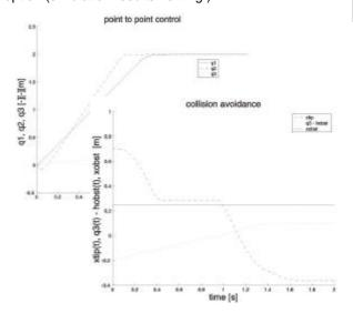
Task c: Collision avoidance: As at MATLAB level no event mechanism is available, for collison handling again voltage was also directly regulated in the function for the right side. In case of emergency, the PD control was used as if the final state was reached permanently, so that only the speed was regulated down. With an if assignment the emergency limits were realised (results see fig. above):
