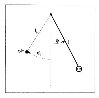
If the pendulum is swinging, it may hit a pin positioned at angle  $\varphi_p$  with distance  $l_p$  from the point of suspension. In this case the pendulum swings on with the position of the pin as the point of rotation and the shortened length  $l_s = l - l_p$ .
