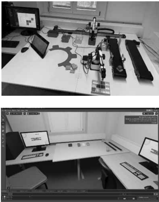
Figure 2: Physical setup and Omniverse implementation.
