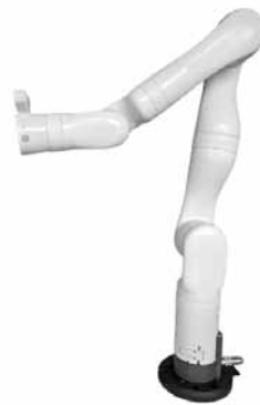
Figure 1: Kinova Gen3 robotic arm [5].
