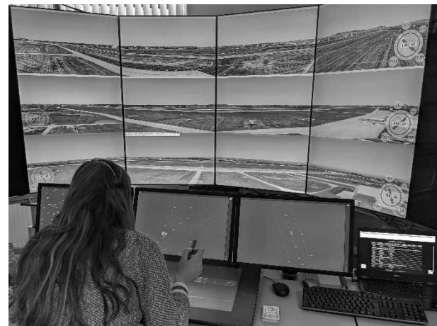
Figure 5: Multiple Remote Tower Setup in the Remote Tower Lab of DLR Braunschweig: One ATCo is controlling three airports, using head-down electronic flight strips and a tower radar display.
