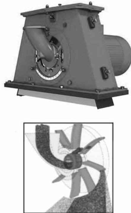
Figure 1: The shot blasting machine and illustration of the principle of operation.
