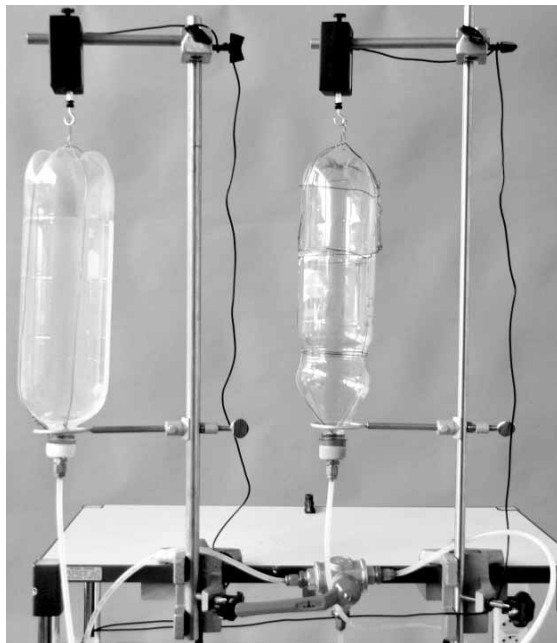
Figure 1: In the first bottle is the air pressurized, the second is under atmospheric pressure.
