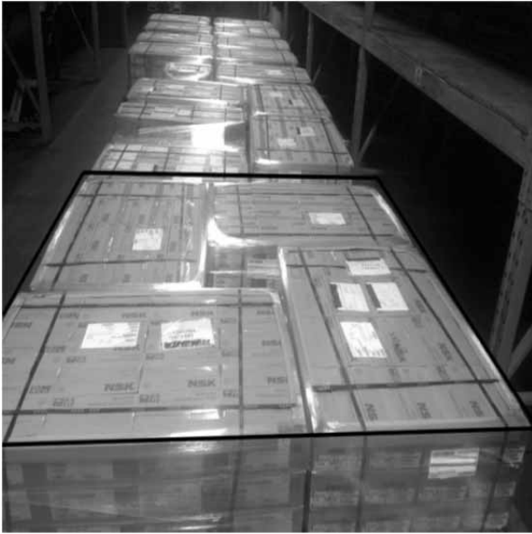
Figure 5. A loader's real-world representation of a loading plan using the same interlocking arrangement.
