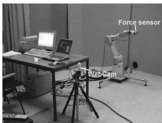
Figure 3. Experimental setup (Mitsubishi PA10, vision system and force sensor)
