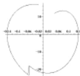
Figure 3: Phase plane curves VL3=dx/dt as a function of IL3=x3
